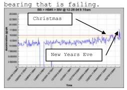
The above plot shows that the blower hit the first alarm on Christmas and the red alarm on New Year's Eve. The remote system watched the progression and sent out E-mails on both occasions. The bearing was replaced shortly after. This example shows another advantage of remote monitoring in that data is taken day, night weekends and holidays.
